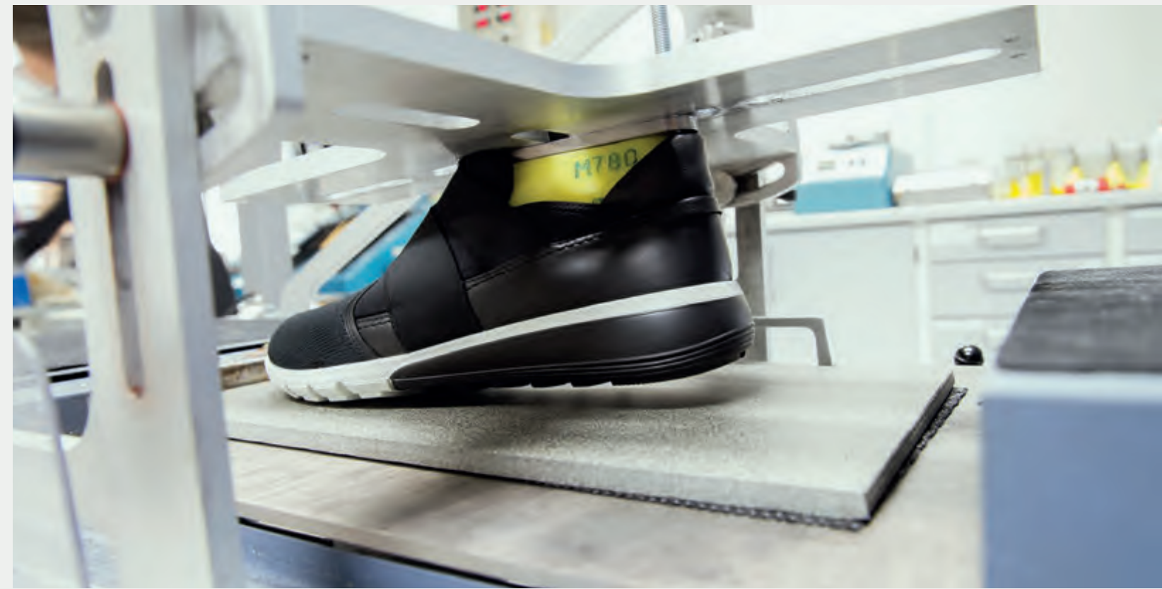
A shoe being tested for slip resistance.
