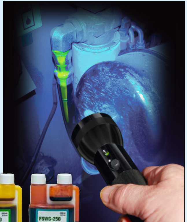
Leak detected using a blue light inspection lamp after the addition of FluidSafe™ additive to the hydraulic fluid system.
