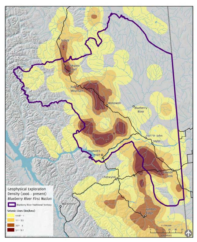
Map 23. Density of seismic exploration (2006-present)
